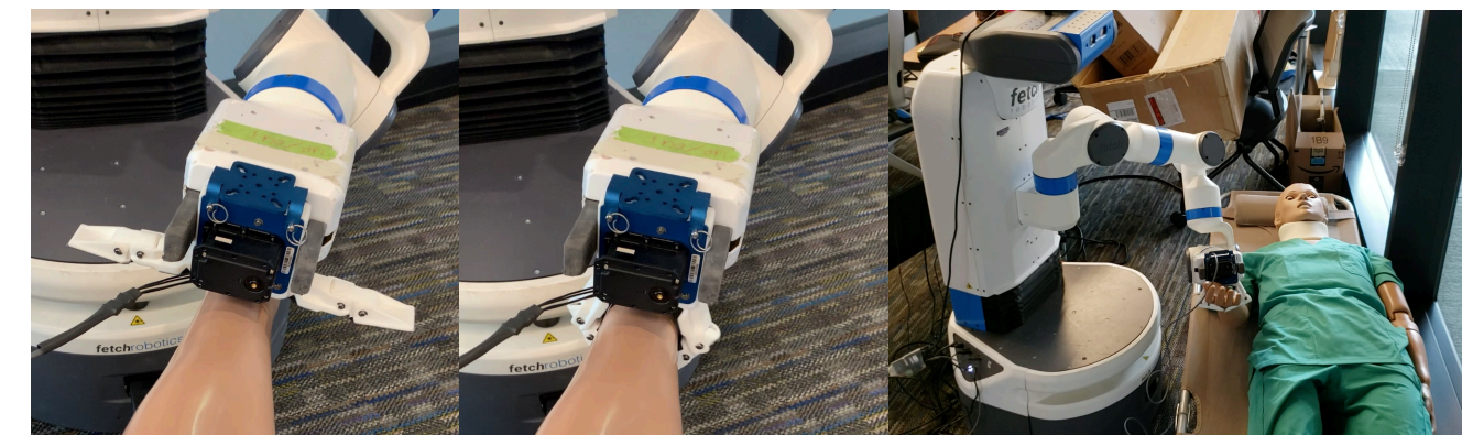
EZGripper™ attached to Fetch is grasping the wrist of the human mannequin.
